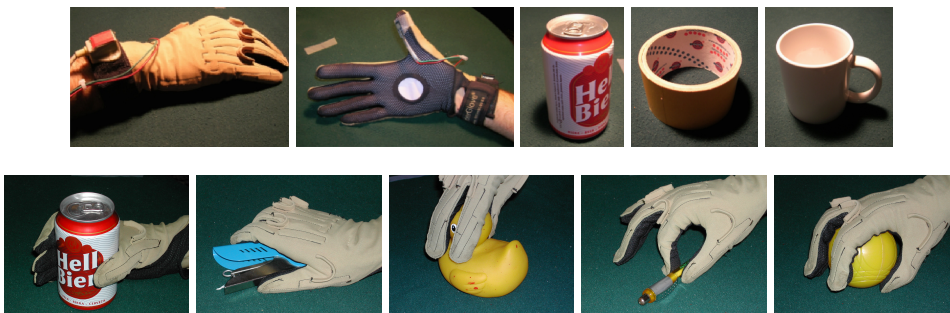
Fig. 6. (above) The devices and some of the objects used for the experiment, left to right: the CyberGlove, the Force Resistor Sensor attached to the subject's thumb, the beer can, the duct tape roll and the mug. (below) The 5 grasp types to be recognized, left to right: power large, power flat, tripodal precision, thumb/index precision and spherical precision.
