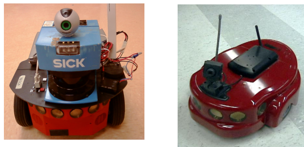
Figure 32 – Pioneer 2DX robots (left) and Amigobot (right) robots used in some of the experiments.
