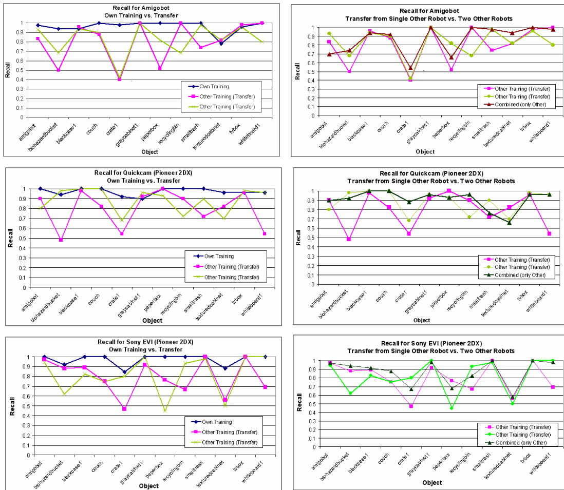
Figure 18 – Object classification results for the three robots and twelve objects in different conditions. Left: Recall rates are shown for all three robots when comparing models learned by the tested robot itself versus models received by one other robot. These figures show large dips in recall rates for certain objects, when compared to the “Own Training” condition. Right: Recall rates are shown for classification of objects given learned models obtained from one other robot (“Other Training (Transfer)”) versus two other robots (“Combined (only Other)”). Combining learned models from other robots resulted in higher average recall.
