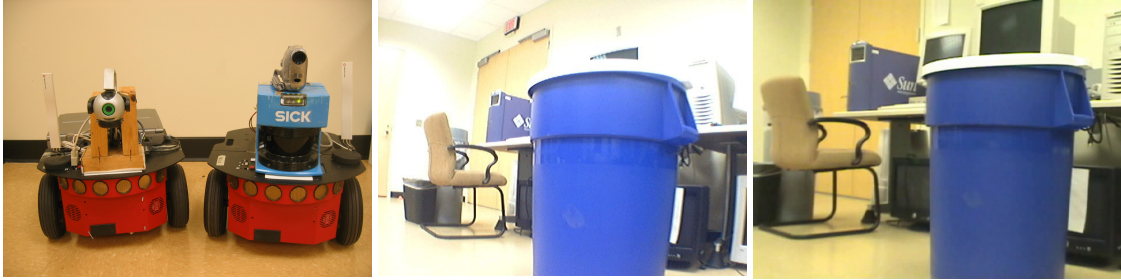
Figure 31 – Pioneer 2DX robots used in some of the experiments (left) and images of the same scene from each robot (middle and right). The middle image is from the robot with the web camera, while the image on the right is from the robot with the camcorder.
