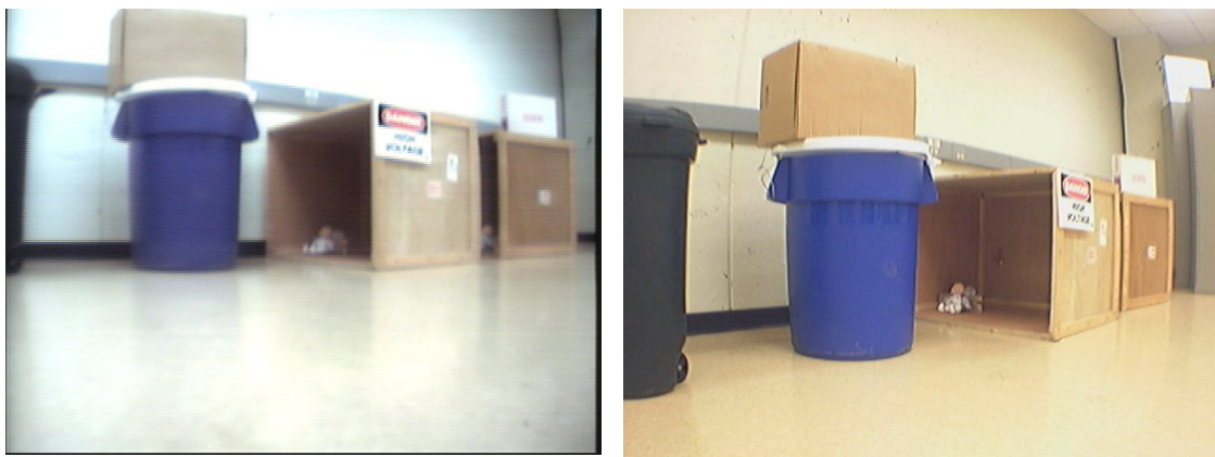
Figure 70 – An example image pair used to calculate the variation of information metric between the two robots. Left: Image from the Amigobot. Right: Image of the same scene from the Pioneer robot.
