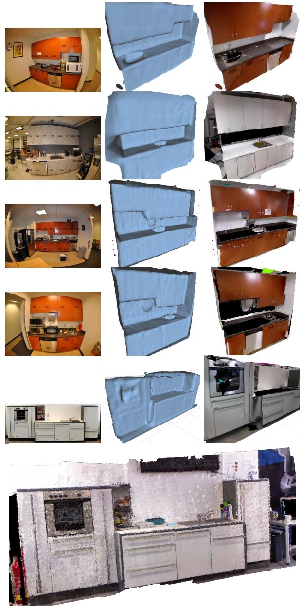
Fig. 5. Left-column : Testbed kitchens at TUM and Bosch RTC. Middle-column : Poisson-based surface reconstruction. Right-column : Blending-based texture re-projection on the left surface mesh. Bottom-row : Data of the TUM kitchen obtained with the handheld Kinect sensor and registered using the RGBD-based registration.
