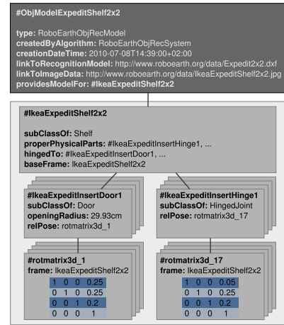
Fig. 5. Object model representation. The object model instance refers to binary data for a model as well as to a detailed description of the object class to be exchanged. In this case, the model describes a cabinet composed of several articulated doors connected with hinges to the cabinet’s frame.
