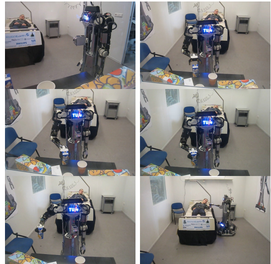
Fig. 1. The Amigo robot performs a mobile manipulation task based on task descriptions, object recognition models and a semantic environment map which it has autonomously downloaded from the RoboEarth database.
