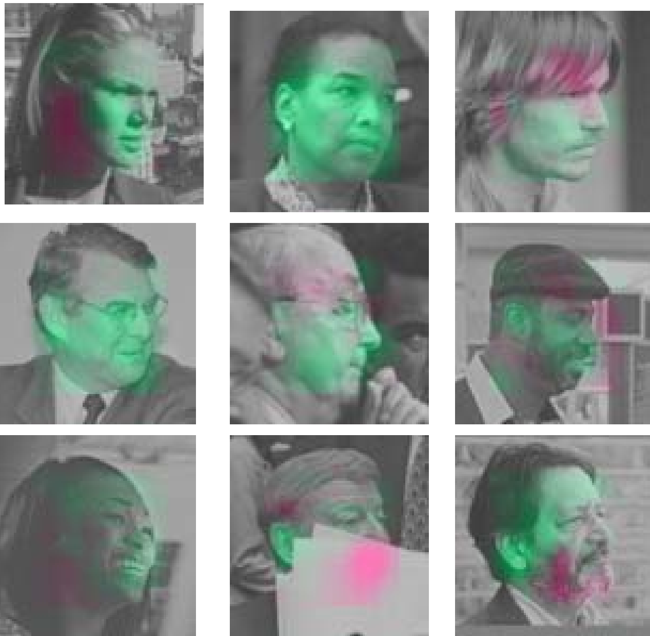
Figure 13b: Positional decomposition of classifier response to particular profile faces. Green areas are “face-like” and red areas are not “face-like.”
