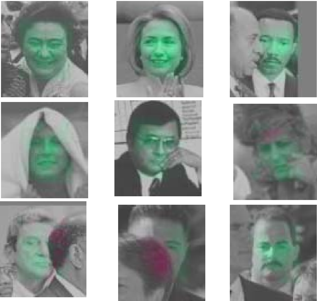
Figure 13a: Positional response of the classifier. Green areas are “face-like” and red areas are not “face-like.”
