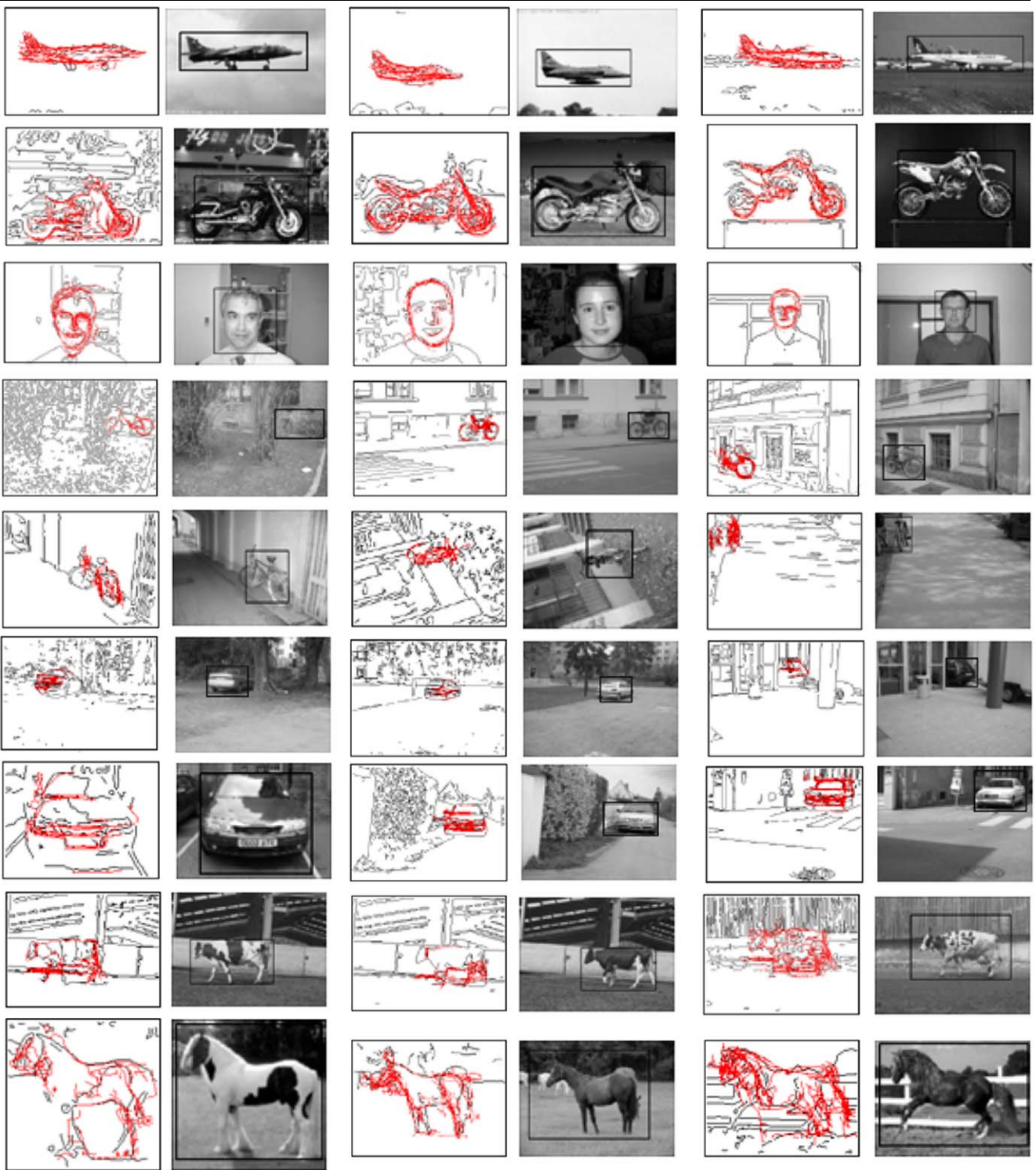
Fig. 31 Examples of detection results using the multi-class detector. On the left we show the matched weak-detectors in red and on the right the resulting detection result as a bounding box
