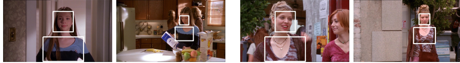
Figure 3: Matching characters across shots using clothing appearance. In the two examples shown the face is difficult to match because of the variation in pose, facial expression and motion blur. The strongly coloured clothing allows correct matches to be established in these cases.
