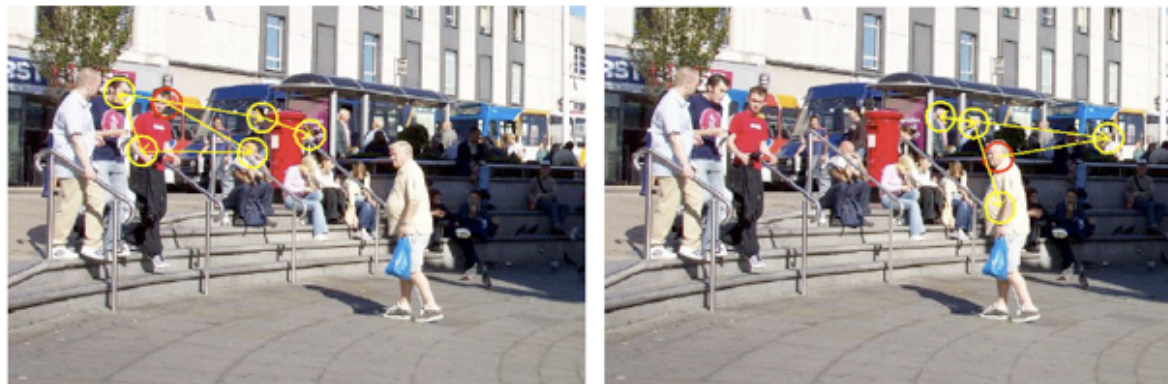
Fig. 7. The trajectories of attention guided by different colour cues. See (left) red colour cue "find a man who is wearing a red T-shirt" and (right) blue colour cue "find a man who is carrying a blue plastic bag".
