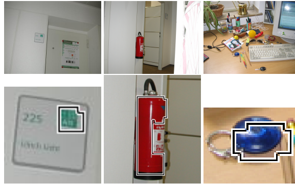
Fig. 18 Top: some training images with targets (name plate, fire extinguisher, key fob). Bottom: The part of the image that was marked for learning (region of interest (ROI)) and the contour of the region that was extracted for learning (most salient region (MSR)) (images from [4]).
