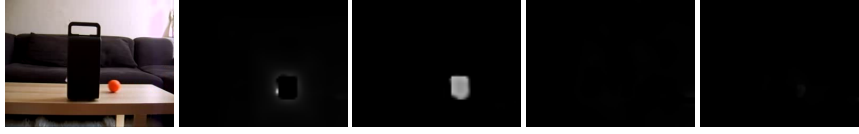
Fig. 11 The motion feature maps M' for a scene in which a ball rolls from right to left through the image. From left to right: example frame, motion maps M'_{\text{right}}, M'_{\text{left}}, M'_{\text{up}}, M'_{\text{down}} .
