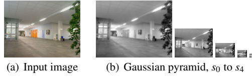
Fig. 6 The image which serves as demonstration example throughout this chapter (a) and the derived Gaussian image pyramid (b).
